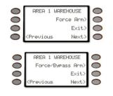
9. Press the appropriate soft key to arm your system with the faulted/bypassed points removed from service.
