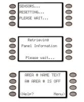
If you enter this function and the detector or sensor resets momentarily, but then returns to a faulted condition, the conditions causing the activation may still be present or the detector may be faulty. Check to be certain that there is no smoke, fire, or other danger present. If you can't reset the detector or sensor contact, your security company.
