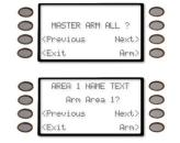
Or press the **Next>** soft key to view each unarmed area and optionally arm each one. To arm a selected area, press **Next>** until the desired area appears (Area name text along with Arm Area # ?). Then press **Arm>**.
