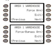
14. Press the appropriate soft key to arm your system with the faulted/bypassed points removed from service.
