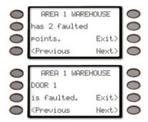
Press Next> soft key repeatedly to scroll through the point text for each faulted point.
