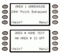
If the bypassed point is a Fire Point, the message *Fire Point Bypassed* begins alternating in the display with *A1 AREA IS OFF*.
