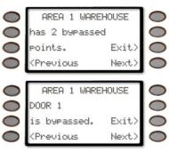
Once the last bypassed point is displayed, the display will change to show the soft key to either force arm the faulted points (*Force Arm>*) or force arm the faulted/bypassed points (*Force/Bypass Arm>*).
