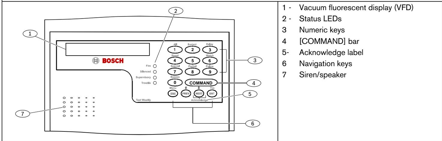
Figure 2: D1256RB Fire Keypad
